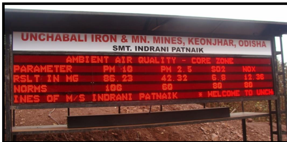
Photo Showing Electronic Display board placed in the mines entrance gate to display the Environmental parameters
