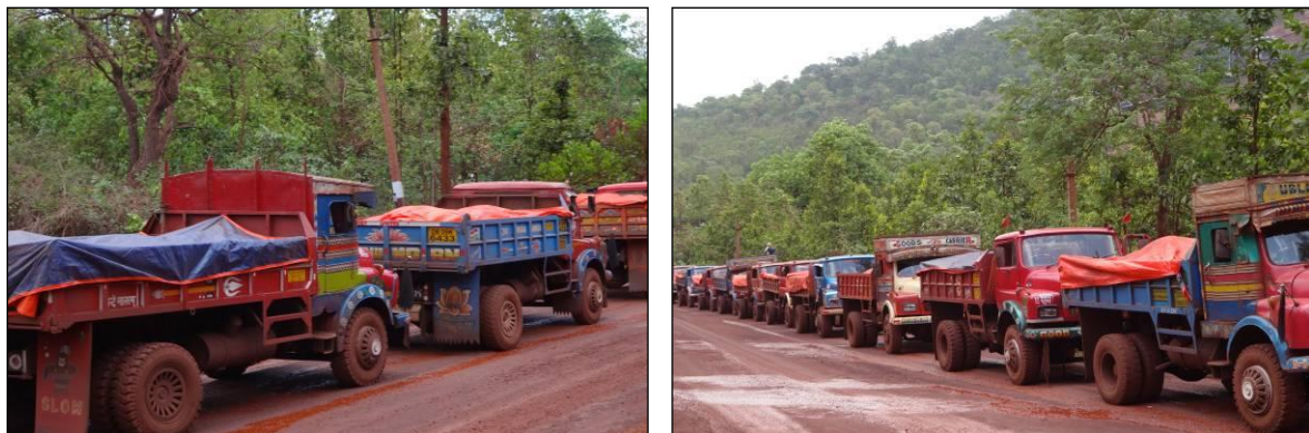
Photo showing transporting vehicles covered with tarpaulin
